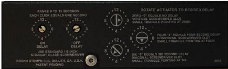
The right side panel has two sections. On the left are two adjustable 16-position rotary switches, one for the On Delay sequence and one for the Off Delay sequence. On the right are three illustrations of how you might set a delay using the rotary switches? The 16 position rotary switches may also be referred to as rotary digital encoders and communicates directly with the microprocessor.
